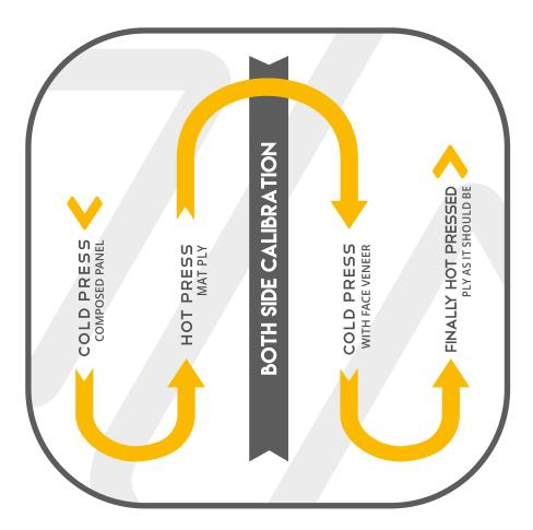
The 4-stage life-cycle gives the plywood an integrated and bonded core with a superbly smooth silky crust. The pre-pressing technology evenly distributes the moisture in the entire sheet ensuring that the final product is of the superior grade. This process injects equal strength and stiffness properties which makes it ideal for applications which demand high strength, stability and rigidity, with a mild pinch of flexibility.
